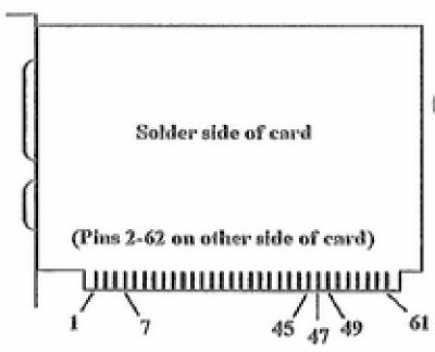
Fig. 1 IBM-PC Comm. Card Pin Numbers count, or use the third column in Table 1 to find your way around. (Note that pins 1 and 61, the first and last on this side, are ground. You should see traces from contacts 47 and 49. These are a couple we will play with.) Also, note that the comm card must have contacts leading to IRQs that you might want to use (contacts 7 and 45, the 4th and 23rd from the flange end, connect to IRQ2 and IRQ5, respectively.)
