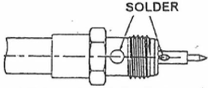
Solder Braid Thru 2 Holes in Body, Solder Center conductor thru Hole. Solder Must Seal Holes For Good Weather Seal
