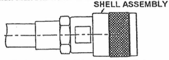
After Cooling, Screw Shell Assembly Onto Body and Wrench Toghten It Tight Against Hex.
