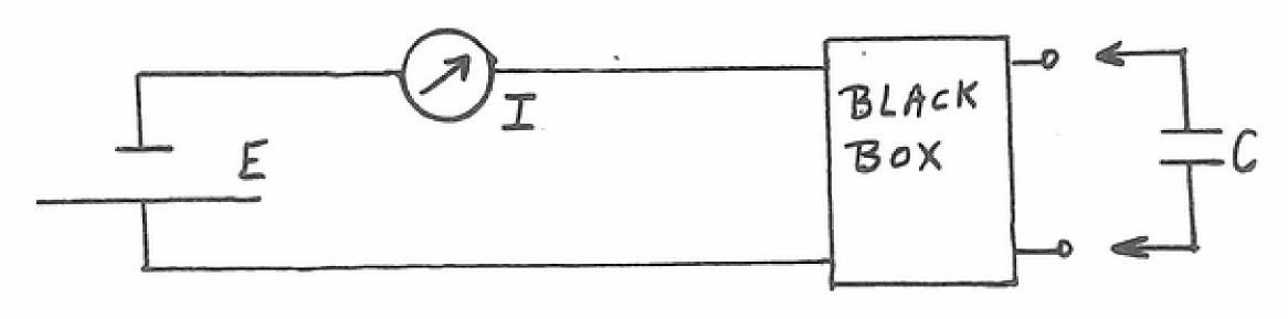
When "C" is connected, "I" is reduced by a factor of approximately 2.
