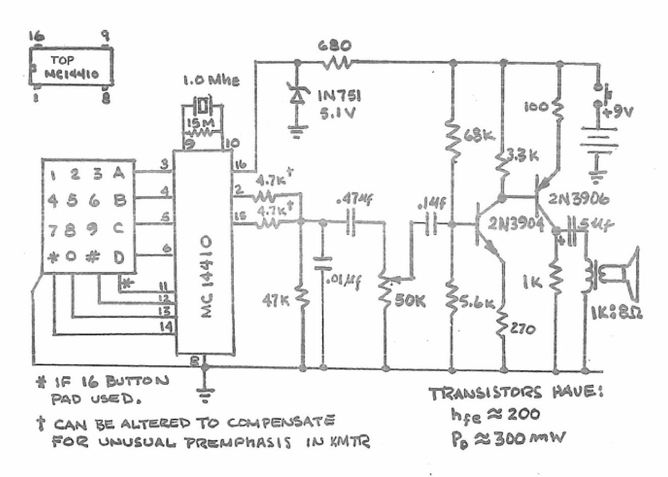
SINCE THE ZENER AND AMP DRAW CURRENT ALL THE TIME, I USED A NORMALLY OPEN PUSHBUTTON TO ENERGIZE THE GENERATOR. THE PLACEMENT OF THIS BUTTON WAS MADE JUDICIOUSLY TO PERMIT "ONE-HAND" DIALING AND SUPPORT. REMEMBER, THE OTHER HAND IS BUSY WITH THE MIKE AND PUSH-TO-TALK SWITCH.
